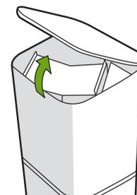
2 Pull up on the plastic card to remove the bag from the canister.
