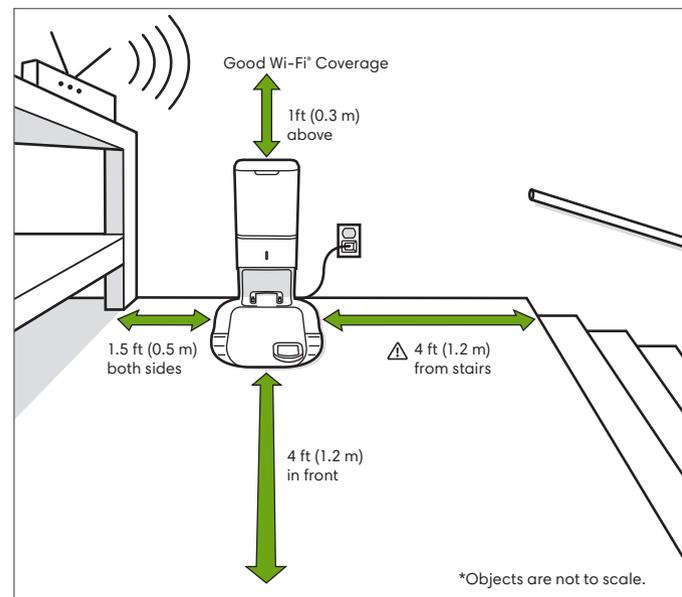
**WARNING:** To prevent the risk of your robot falling downstairs, ensure that the charging station is placed at least 4 feet (1.2 meters) away from stairs.
