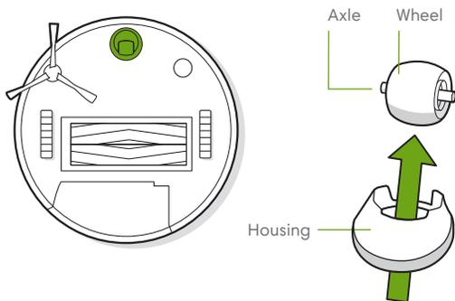
**\* Important:** A front wheel clogged with hair and debris could result in damage to your floor. If the wheel is not spinning freely after you have cleaned it, please contact Customer Care.
