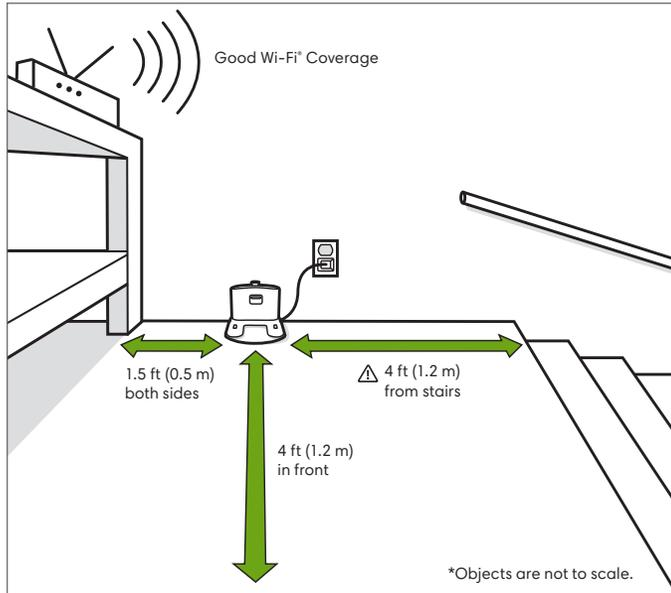
**⚠ WARNING:** To prevent the risk of your robot falling downstairs, ensure that the charging station is placed at least 4 feet (1.2 meters) away from stairs.
