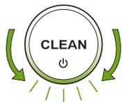
When the robot senses its bin needs to be emptied, the light ring indicator will illuminate in a red sweeping motion toward the rear.
