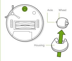
Important: A front wheel clogged with hair and debris could result in damage to your floor. If the wheel is not spinning freely after you have cleaned it, please contact Customer Care.
